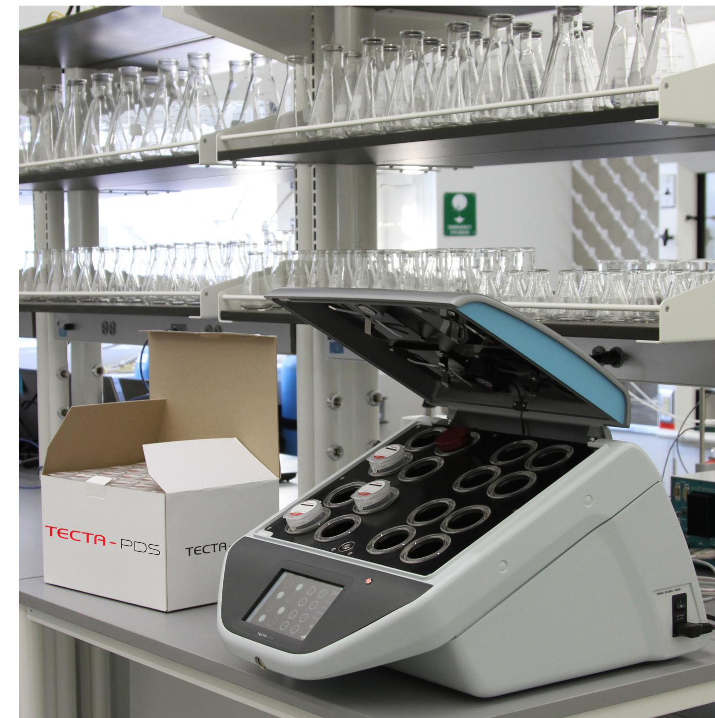
TECTA B16 instrument and TECTAlert cartridge schematic
